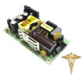
60W Open frame type switching power supplies for Medical Equipment
