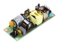
The SBU31 series of products, open frame constructed, AC/DC switching mode power supplies provide 30 Watts of continuous output power. They are suited for use in portable equipments and many other applications. All models meet CISPR-22 class B emission Limits and are designed to comply with new CE requirements. All units are 100% burned in and tested.
