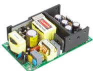
The SBU151 series of compact, open frame constructed, AC/DC switching mode <a href="mailto:power">power</a> supplies provide 150 Watts of continuous output power. They are suited for use in based systems, portable equipments and many other applications. All models meet FCC Part-15 class B and CISPR-22 class B emission Limits and are designed to comply with UL/c-UL(UL 60950-1:2nd Edition) ,TUV/Bauart(EN 60950-1:2nd Edition) and new CE requirements. All units are 100% burned in and tested.
