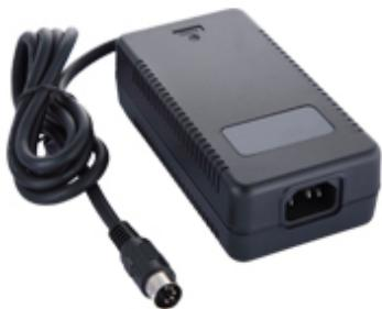
The SPU80 series of AC/DC switching mode power supplies provide 80 Watts of continuous output power. All supplies are UL 94V-1 min compliant. All models meet FCC Part-15 class B and CISPR-22 class B emission Limits and are designed to comply with UL/c-UL(UL 60950-1:2nd Edition), TUV/GS(EN 60950-1:2nd Edition) and new CE requirements. All units are 100% burned in and tested.
