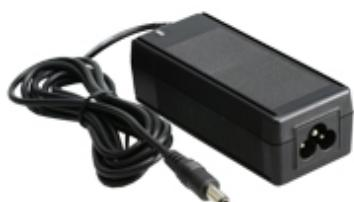
The SPU25C series of AC/DC switching mode power supplies provide 25 Watts of continuous output power and is well-suited for a variety of applications. All supplies are UL 94V-1 min compliant. All model meet FCC Part-15 class B and CISPR-22 class B emission Limits and are designed to comply with UL/c-UL(UL 60950-1:2ndEdition), TUV/GS(EN 60950-1:2ndEdition) and new CE requirements. All units are 100% burned-in and tested.
