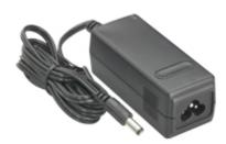
The SPU16C series of AC/DC switching mode power supplies provide 15 Watts of continuous output power and is well-suited for a variety of applications. All supplies are UL 94V-1 min compliant. All model meet FCC Part-15 class B and CISPR-22 class B emission Limits and are designed to comply with UL/c-UL(UL 60950-1:2ndEdition), TUV/GS(EN 60950-1:2ndEdition) and new CE requirements.
