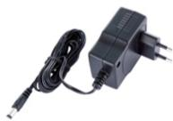
The SPU12C series of AC/DC switching mode <u>power</u> supplies provide 15 Watts of continuous output power. All supplies are UL 94V-1 min compliant, include a 2 prong plug-in mains connector for certain applications. All models meet CISPR-22 class B emission Limits and are designed to comply and new CE requirements. All units are 100% burned in and tested.
