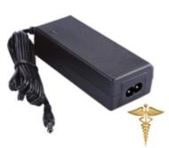
The HPU63B series of AC/DC switching mode power <sup>™</sup> supplies provide 63 Watts of continuous output power. All supplies are UL94V-1 min compliant. They are suited for use in Health care applications. All models meet FCC Part-18 class B and CISPR-11 EN55011 class B emission Limits and are designed to comply with ANSI/AAMI ES 60601-1: 2005(UL/cUL 3rd Edition), EN 60601-1:2006 (TUV/T-mark 3rd Edition) and new CE requirements. All units are 100% burned in and tested.
