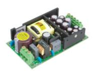
63W Open frame type Extreme operating temperature power dsupplies
