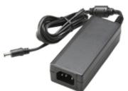
The EPU60A series of AC/DC switching mode <u>power</u> supplies provide 60 Watts of continuous output power. All supplies are UL 94V-1 min compliant. All models meet FCC Part-15 class B and CISPR-22 class B emission Limits and are designed to comply with UL/c-UL(UL 60950-1:2nd Edition), TUV/GS(EN 60950-1:2nd Edition) and new CE requirements. All units are 100% burned in and tested.
